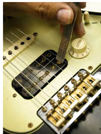
Above, right A flame-maple Telecaster neck hits the buffing wheel; measuring polepiece height
