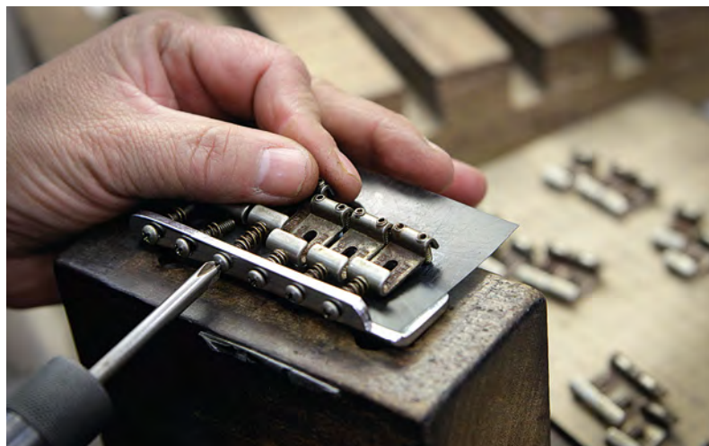
Above, left Master Builder Paul Waller in action; a collection of exotic Strat necks await the next stage; a Relic Stratocaster bridge is hand-assembled
